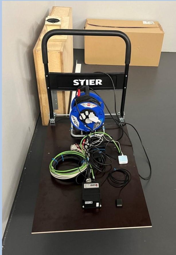
Figure 1: Prototype with Inertial Sensors + GNSS. Sourc: THI
