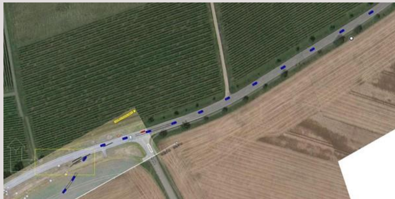
Figure 3: Reconstruction of a single-vehicle accident based on the EDR data sets with the PC-Crash software. Source: THI
