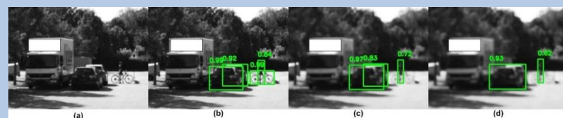
Fig. 3: Illustration showing (a) original scene with two cars, person and bicycle at \approx 40 meter and objects detected by F-RCNN model for image captured at (b) 0 \mu\text{m} defocus (c) -30 \mu\text{m} defocus and (d) -40 \mu\text{m} defocus. A decrease in confidence score and increase in false negative with increase in defocus is seen.
